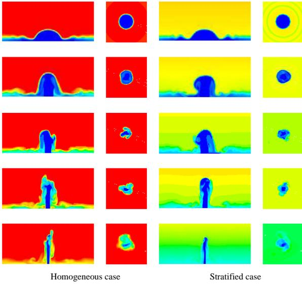
Figure 4: Steady-state temperature contours of fountains at  $Re = 200$  with varying  $Fr$  in both a homogeneous fluid and a linearly stratified fluid at  $s = 0.03$ . The first and third columns are temperature contours in the vertical plane through the symmetry axis of the cylinder, and the second and the fourth columns are temperature contours in the horizontal plane at height  $Z = 0.5Z_{m,i}$ . The top to the bottom rows correspond to  $Fr = 1, 2, 3, 5$  and  $8$ , respectively.
